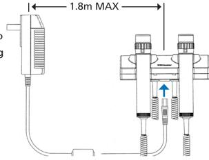
For the Gen Med Wall Units drill two holes Ø6mm x 55mm deep and 110mm apart.
